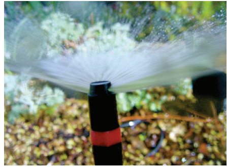
Fig 7: A typical pop-up sprinkler head when not in use (left pic) and when in operation (right pic).
