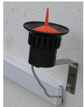
Fig 9: A common rain sensor, an accessory of an irrigation system.
